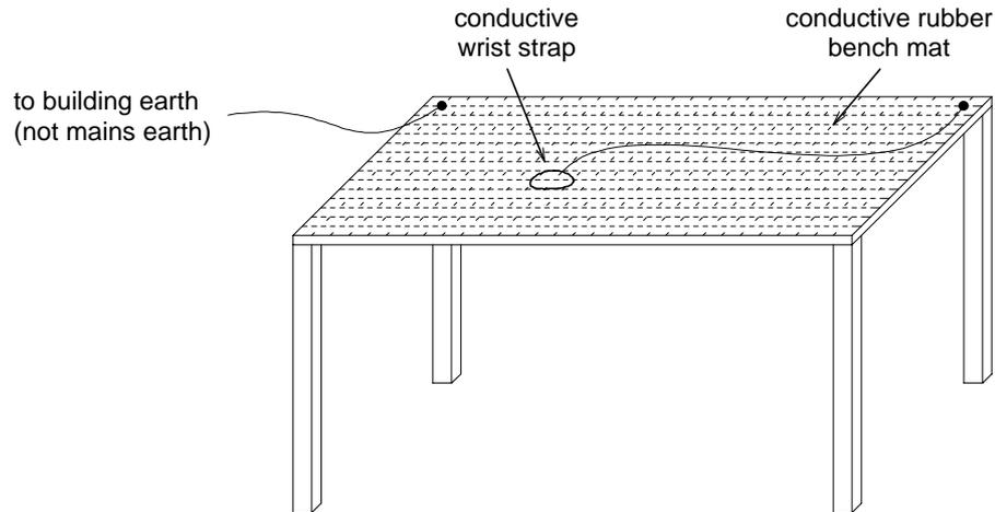
*Figure 1.2 Typical Anti-static Bench Set-up*
