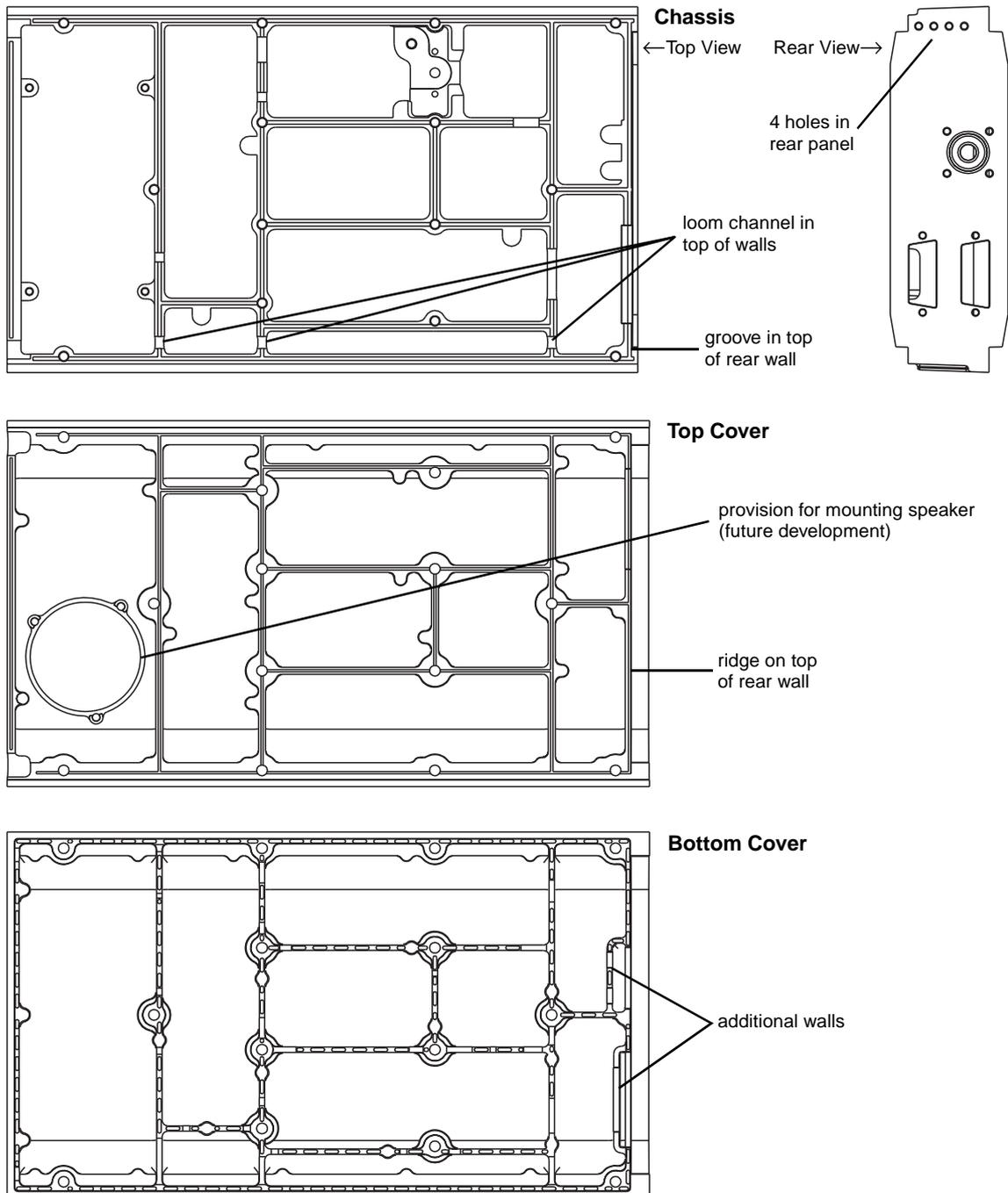
Figure 2.4 Identification Of New-Design Chassis & Covers
