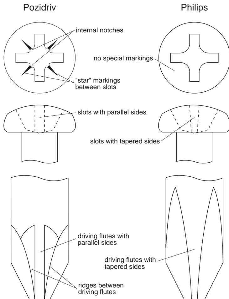
**Figure 2.2** Pozidriv & Philips Screw & Screwdriver Identification
